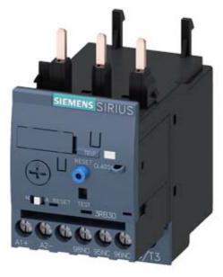
Overload relay 3...12 A for motor protection size S0, CLASS 10E contactor mounting Main circuit: screw term. Aux. circuit: screw term. Manual/Auto RESET
